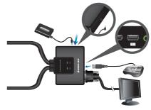
Connect a powered USB hub to the console mouse port, then connect the mouse to any available USB port in the hub. Then, connect any peripherals that you want to share between your computers to the other available USB ports in the hub.
